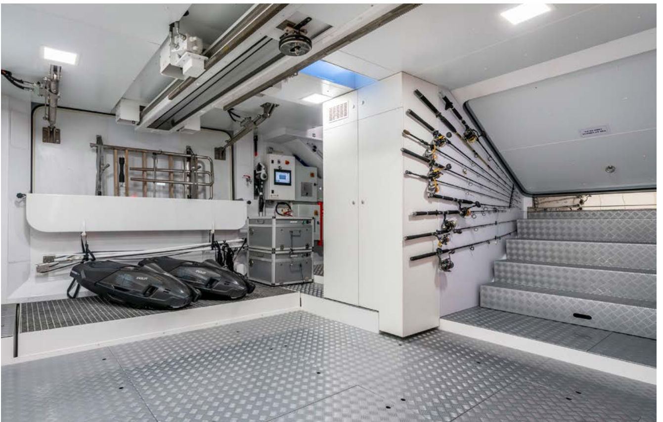
LAZARETTE, STARBOARD SIDE / SHELL DOOR AND CEILING-CRANE
