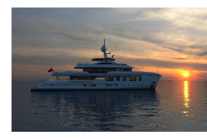
With a robust steel hull and a **total length just above 43m and a generous beam of 8.60m**, Deep Blue 141 has a Gross Tonnage shy of **500GT**. Propelled by twin Caterpillar **C32 engines delivering 746kW** each, she will reach a top speed of 15.3 knots. One of the standout features of this explorer yacht is her impressive **range** of around **7 500 nm at 10 knots**, a testament to her capabilities for global exploration.
